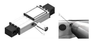
Lubrication is effected by an oiled felt insert. The felt can be re-oiled through lubrication nipples attached laterally to the ends of the roller packs.
